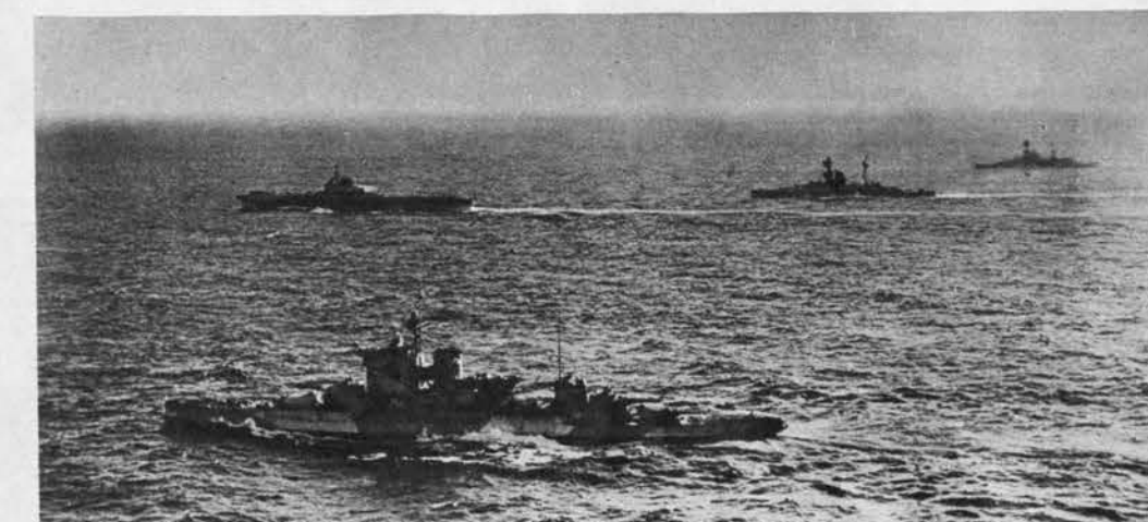
Warspite ( foreground ) is typical British ship with blockhouse bridge, low straight stack, balanced design. Sister ships Resolution and Royal Sovereign ( right ) are distinguished by tall mainmasts.
